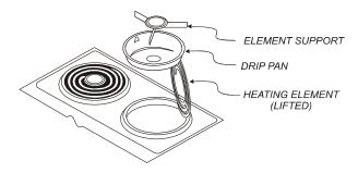
Fig. 7 Hotplate Drip Pan Installation
